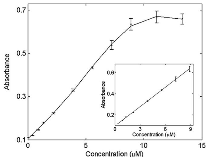
Fig. 2. Absorbance value at 800 nm versus  $\text{Hg}^{2+}$  concentration. Experimental conditions:  $c_{\text{NaCl}} = 53.3 \text{ mM}$  and  $c_{\text{TBA}} = 260 \text{ nM}$ . Inset: derived calibration curve.
