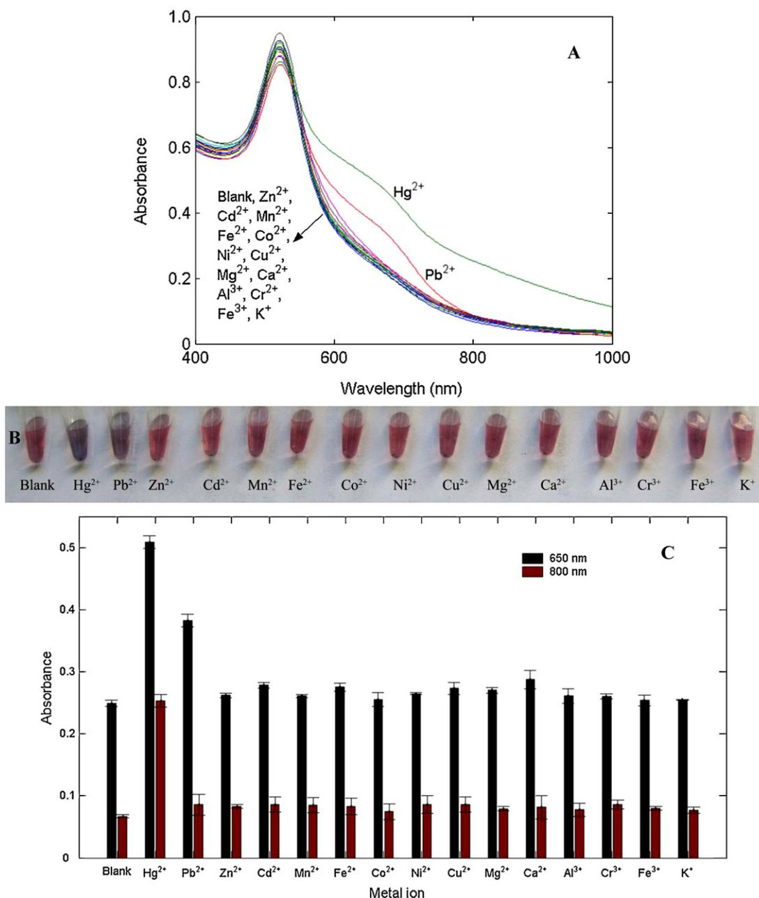
**Fig. 1.** (A) Absorption spectra of the AuNP solution mixed with 180 nM TBA in the absence (blank) or presence of 5.56  $\mu\text{M}$  various metal ions after the addition of 40 mM NaCl. (B) Visual color changes upon treatment of the TBA/AuNP system with or without (blank) various metal ions in the presence of NaCl. Experimental conditions are as in (A). (C) Selectivity of the analysis of  $\text{Hg}^{2+}$  at 650 nm and 800 nm. Experimental conditions are as in (A).
